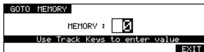
To locate to a previously stored locate memory, press GOTO, F6 (MEMORY) and enter the appropriate memory number 0-99 using the track keys (ALL/0, 1-8, SYNC/9) as a numeric keypad. Finally, press ENTER (see STORING LOCATE MEMORIES).
