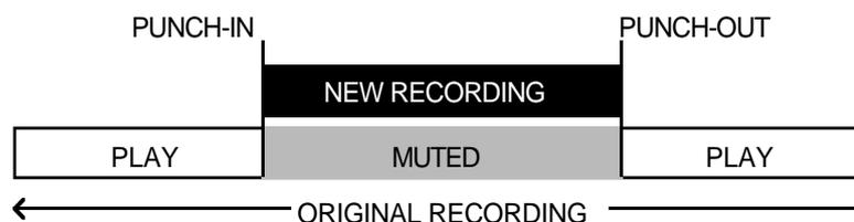
*This means that in most cases, the DD8 will drop in and out of record pretty much like a normal MTR. Usually, on most hard disk recorders, due to disk speed restrictions and SCSI bandwidth, there is a gap of several seconds or more at the point of drop-out. This is not so on the DD8 and it is possible to punch in and out seamlessly on mono and stereo tracks.*
