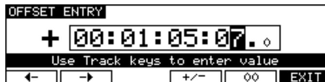
Soft keys F1 and F2 can be used to move the cursor to the sub-frame field, or any of the other fields. The offset time is then entered using the track keys as a numeric keypad or the current digit can be nudged using the DATA +/- keys.
