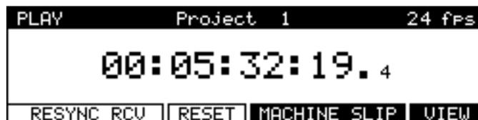
The top line of the screen shows the name of the current Project, as well as the current frame rate.
