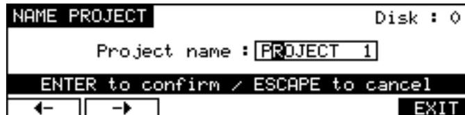
Use the F1 (<-) and F2 (->) keys to move the cursor to the left/right. Use the DATA +/- keys to scroll through the available characters in order to set the name for the new project. When you are finished, press ENTER to set the new project name.
