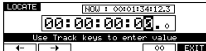
You may locate to a timecode position by pressing GOTO followed by F5 (LOCATE). Use the track keys as a numeric keypad to enter the required time. Values enter from the right and time divisions (i.e. hours, minutes, seconds and frames) are confirmed using the 00 'double zero' soft key (F5).
