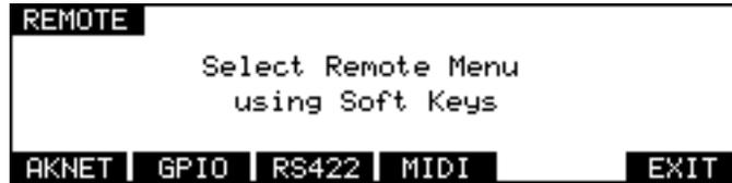
Soft keys are only shown for the installed option boards. If certain boards are not installed, they will not be detected by the DD8 and their keys will not be shown here.
