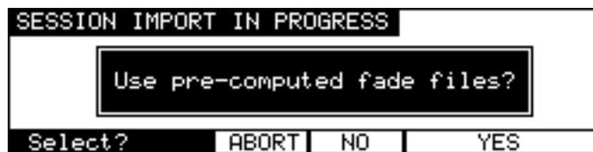
If you select YES, the DD8 will load and playback all fade-regions from the rendered fade files on disk. If you have created any custom fades in Protools, you should choose this option to ensure the DD8 plays back the file correctly.
