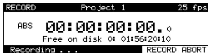
Pressing RECORD ABORT (F5/F6) aborts the recording process. To stop recording, press STOP. To drop out of record (i.e. stop recording but keep playing), simply press PLAY - the DD8 will drop out of record and keep playing.
