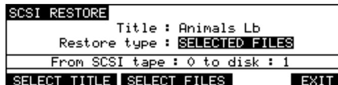
The easiest restore to perform is when a tape has just one backup on it. In this case, simply select ALL PROJS & LIBS and press ENTER. Regardless of the type of backup you performed on this tape, any projects and libraries found on the tape will be restored.
