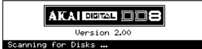
The DD8 will look at the disk drives attached to the system. If a disk containing a valid PROJECT is found, it will be loaded automatically and you will see the main playback screen:
