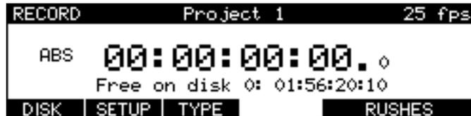
The top line of the screen shows the name of the current Project, as well as the current frame rate. Pressing DISK (F1) takes you to the Record Disk page :
