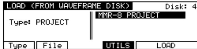
Pressing TYPE (F1) will move the cursor to the file type field where you can select the type of file you want to load. Normally, this should be left on PROJECT to view the available projects on the disk. ALL FILES can also be selected to view a list of all the files on the disk.
