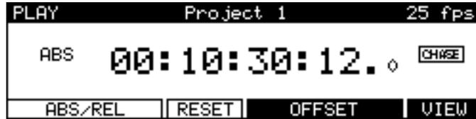
When the DD8's internal time is at the same position as the external time (and the sample rate is synchronised to the speed of the external time source), the CHASE display will change to LOCK.
