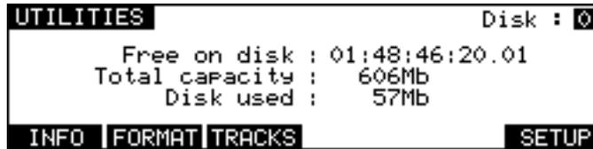
Some files created by Macintosh applications may contain more than 8 tracks of audio. In this case, you may wish to use several DD8s to playback the audio with up to 8 tracks playing from each machine. Pressing the TRACKS key (F3) on the UTILITIES page will take you to the IMPORT TRACKS page which can be used to select the 8 tracks that will be imported:
