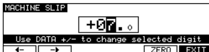
This page allows you to slip the DD8's time with respect to the biphase machine. F1 and F2 are used to move the cursor to the correct position (frames or sub-frames), and the DATA +/- keys are used to adjust the value. Note that the Sub-Frame value (1/10th frame, 1/4th frame, 1/2 frame) depends on the setting in SYSTEM/DISPLAY (10th Frame, Film Perfo, Video Field). The ZERO key (F5) resets the offset to zero.
