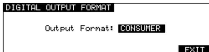
In this page, the OUTPUT FORMAT field allows you to set the format for the digital outputs of the IB-D8MA24 board and you may choose PROFESSIONAL or CONSUMER. PROFESSIONAL would be the choice to make when interfacing with AES/EBU digital audio equipment whilst CONSUMER would be the choice when connecting to DAT machines that use the SPDIF format of digital inputs.
