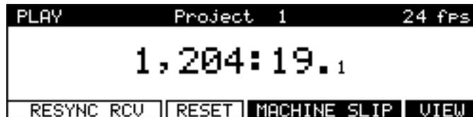
The top line of the screen shows the name of the current Project, as well as the current frame rate of the timecode display.
