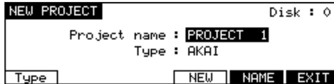
Pressing NEW (F4) will create a new Project (using Flash ROM settings), with the name shown in the Project Name field. After creating a new project, the DD8 will go to Record Mode ready to make new recordings.
