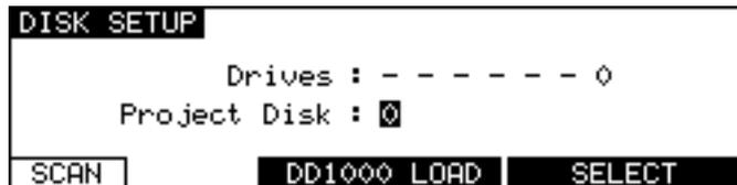
To load a DD1000 Qlist, you should press the DD1000 LOAD key (F3/F4) to go to the LOAD DD1000 QLIST page. The screen will show a list of DD1000 Qlists which you may load as normal.
