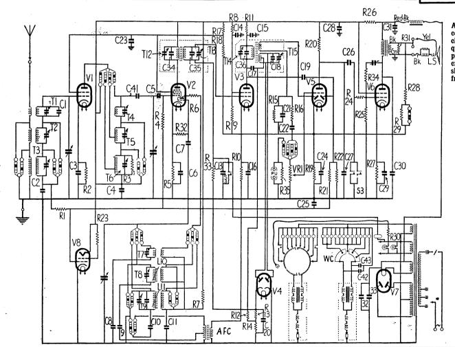
A motor-tuned receiver, this model includes automatic frequency correction provided by V4, a discriminator valve. By shifting the oscillator frequency, this puts
