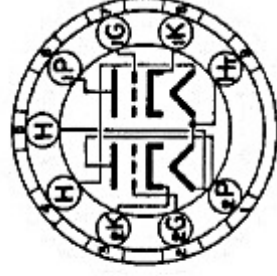
BOTTOM VIEW SMALL BUTTON 9 PIN BASE
