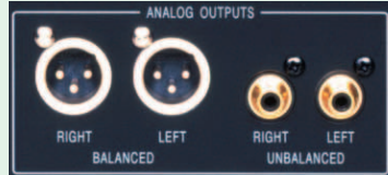
Balanced and unbalanced analog output connectors
