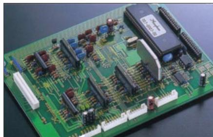
■ Assembly with DA1 encoder/decoder, ultra jitter-free PLL circuit, and other digital processing circuits. Two MDS D/A converter boards (one each for right and left) use Teflon with a low dielectric constant and low loss. The analog output connector assembly is also visible.
