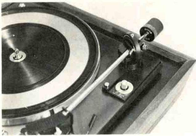
Fig. 1 —Most adjustments are found near the arm mounting—coarse and fine counterbalance, stylus force, anti-skating, and tonearm cueing height. Note record spindle for single-play use—it rotates with the platter to avoid wearing the center hole and to ensure concentricity.
