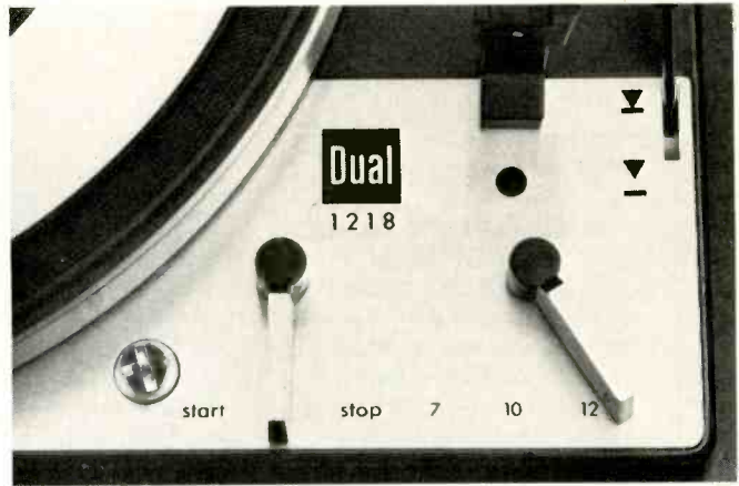
Fig. 3 —The right front of the chassis accommodates the three most-used operating controls—the cueing lever, which extends out of the photo at the upper right, the record-size selector with positions for 7-, 10-, and 12-in. records, and the start-stop lever. The hole above the record-size lever gives access to an adjustment for the set-down position for 12-in. records.
