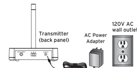
**Note:** There is no transmitter ON/OFF switch. The transmitter is designed to be left plugged in and powered at all times. If you will not be using the AW827 for an extended period of time, unplug the transmitter AC power adapter.
