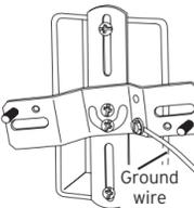
5. Find the copper ground wire coming from the wireless speaker. Twist it together with the ground wire coming from the outlet box.
