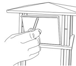
1. Use a small flat tool (like a flat-head screwdriver) to open the top of the lantern's front door.
