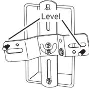
3. Mount the crossbar to the outlet box using the mounting screws included in this package.
