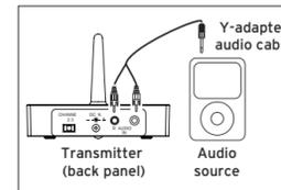
1. Plug the stereo plugs on the provided Y-adaptor audio cable into the AUDIO IN jacks on the back of the transmitter (make sure to match the colors on the plugs and jacks).
