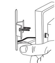
1. Make sure power is off for the outlet box at the main circuit breaker.
