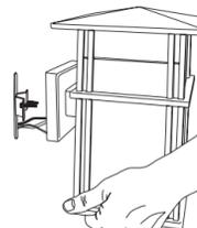
8. Place the wireless speaker onto the two side screws on the crossbar. Secure the speaker onto the wall with the two caps included in this package.
