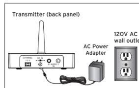
3. Connect the small, round plug from the transmitter AC power adapter to the transmitter's DC IN jack. Plug the other end of the transmitter AC power adapter into any standard 120V AC wall outlet.
