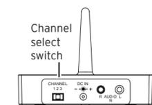
2. Set the channel select switch on the back of the transmitter to one of the transmitter's three broadcast frequencies: 1, 2 or 3. If you experience poor reception or interference, try choosing a different frequency by moving the channel select switch to another position.
