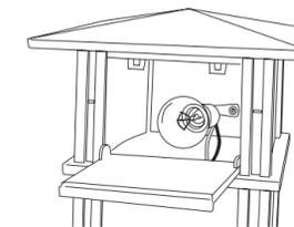
2. Insert the bulb and screw it into the base.
