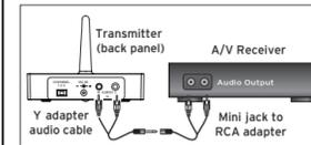
2. Plug the mini-plug end of the provided Y-adaptor into the mini-jack to RCA adapter.
