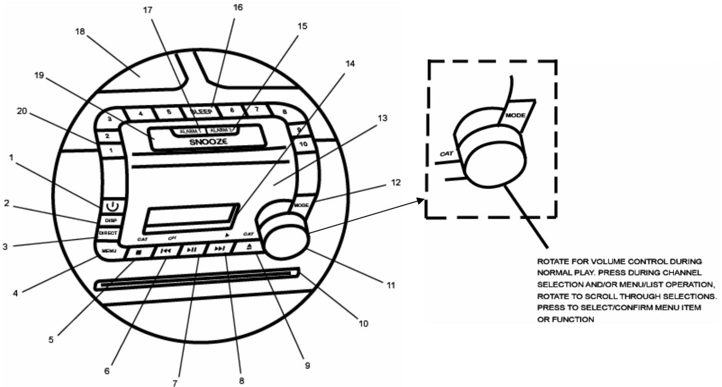
ROTATE FOR VOLUME CONTROL DURING NORMAL PLAY. PRESS DURING CHANNEL SELECTION AND/OR MENU/LIST OPERATION, ROTATE TO SCROLL THROUGH SELECTIONS. PRESS TO SELECT/CONFIRM MENU ITEM OR FUNCTION
