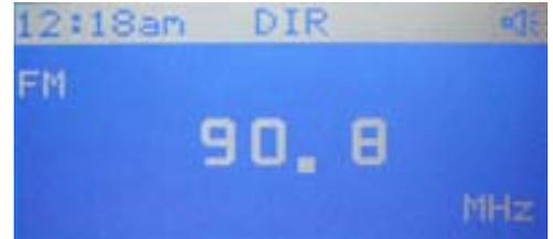
Press DIRECT button to preset A, B, C, and hold number button (1-10) over 3 seconds to store station frequency in memory bank A
