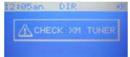
If the XM antenna is not connected, or an XM antenna fault occurs, the following message screens may appear:
