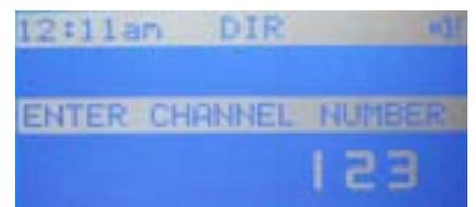
**Note:** After 20 seconds, channel scroll will time out and the scroll wheel will return to Volume Control.
