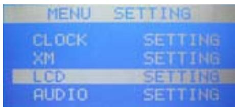
Press CH+/- to highlight this item; then press select. Adjust contrast range using CH+/-
