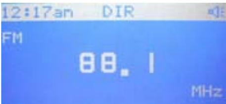
In FM mode, press CH+/- to change channel frequency in 100kHz steps.
