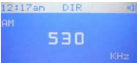
In AM mode, press CH+/- to change channel frequency in 10kHz steps.
