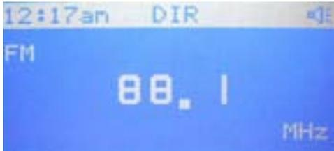
Press the CH +/- buttons to change FM frequency in 100kHz steps; press select
