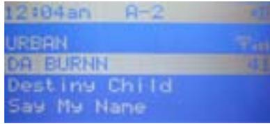
Press and hold DIRECT to access preset channel list in memory bank A; press CH Up or Down to scroll through selection.
