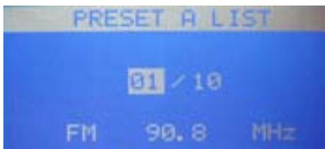
Press and hold DIRECT button over 3 seconds to display list of stored frequencies in current bank. Press the CH Up or 7 preset Down buttons to scroll through selections
