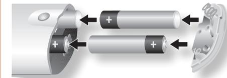
2. Insert four 'AAA' batteries into the battery compartment – two facing the top of the unit, and two facing the end, as in the diagram.
