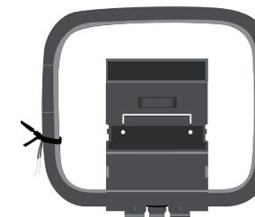
1. Release the tie-wrap and unwind the twisted lead. Fold the plastic stand forward through the loop frame.
