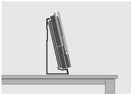
**Fig. 6:** The BeoSound 9000 placed in a near upright position on a level surface, e.g. a table or shelf. When BeoSound 9000 is placed like this, the CD mechanism must be centred for a horizontal position.
