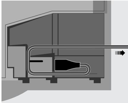
*For safety reasons fasten the mains cord as shown, before running it out from the socket compartment.*
