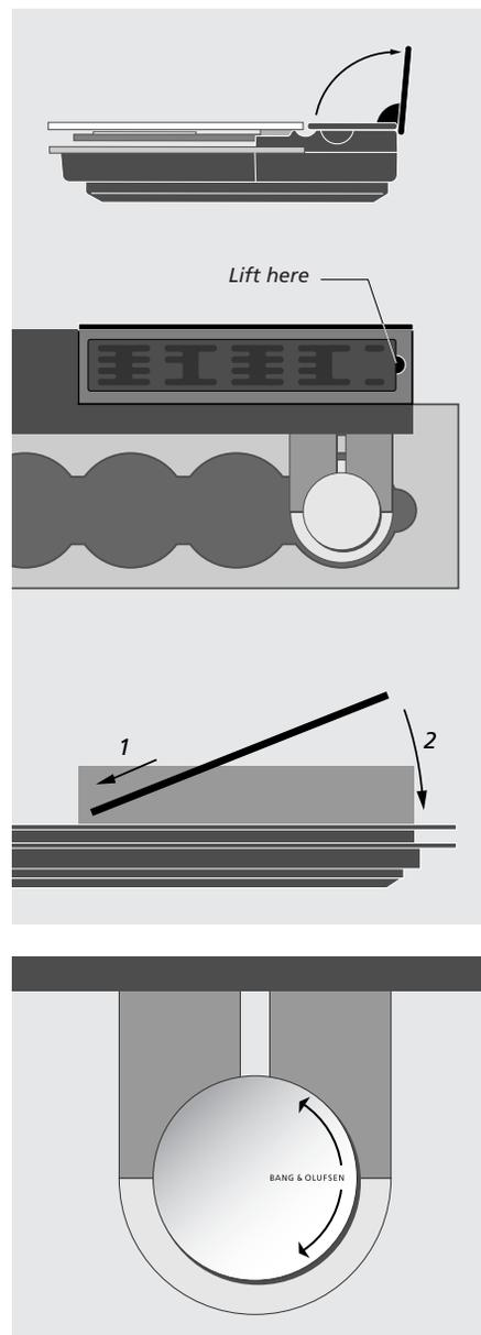
*You can rotate the CD clamping lid (with the Bang & Olufsen name) in order to ensure that the name always appears in a horizontal position (and not upside down).*
