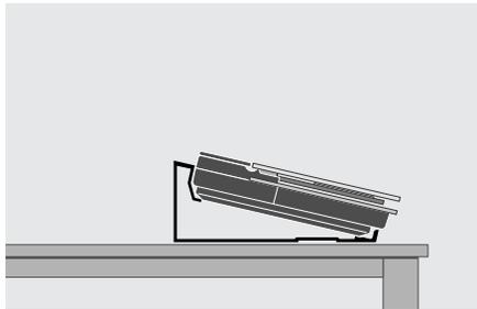
**Fig. 5:** The BeoSound 9000 placed in a slant position on a level surface, e.g. a table or shelf. When BeoSound 9000 is placed like this, the CD mechanism must be centred as for a flat position (factory setting).
