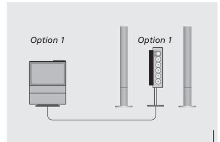
*In a one-room AV integrated setup, a pair of active speakers has been connected to the BeoSound 9000.*
