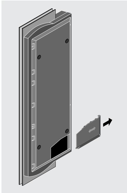
Remove the cover in the bottom plate of the BeoSound 9000 to gain access to the sockets. The socket compartment contains the socket for the mains cord.
