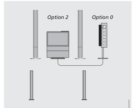
*In a fully integrated system, your BeoSound 9000 acts as a mere audio source. The sound is reproduced through the speakers in the BeoVision TV – or, as shown here, through a set of active speakers connected to the TV.*
