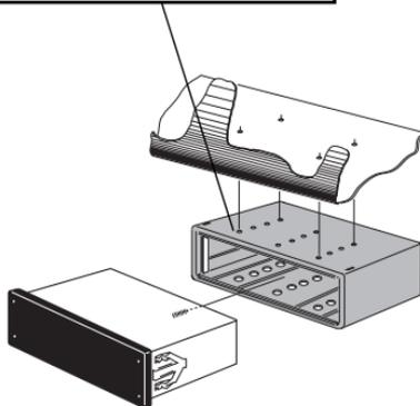
Spacer installation frame 6 mm
