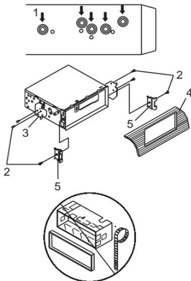
Fixing the equipment to the standard radio mounting clip.
