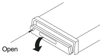
2. Pull off the front cover towards the front of the unit by pressing down on the release zone.
