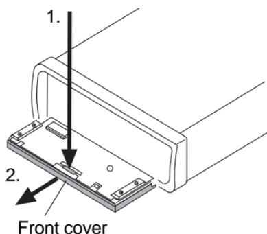
3. Put the front cover in the supplied case for safe keeping as soon as you have removed it.
