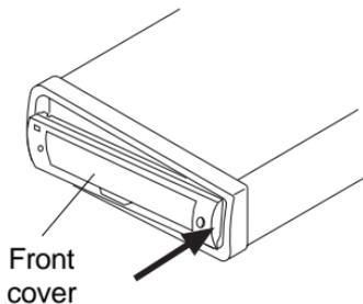
2. Note that if the front cover is inserted incorrectly, the operating controls may not function correctly, and that parts of the LCD display may not appear. Press the **OPEN** button, and reinsert the front cover.
