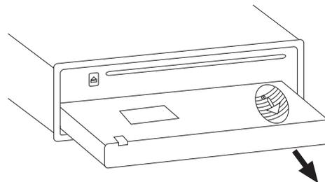
➡ Hold the control panel by its right side and then pull it **straight** out of the bracket.
