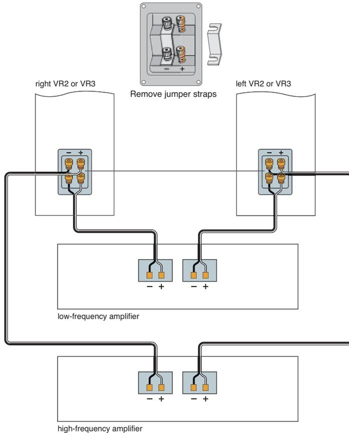
**CAUTION:** Do not use an external active crossover with your VR speakers. The external crossover and the VR's internal crossover can interact and distort the phase and frequency response of the system.
