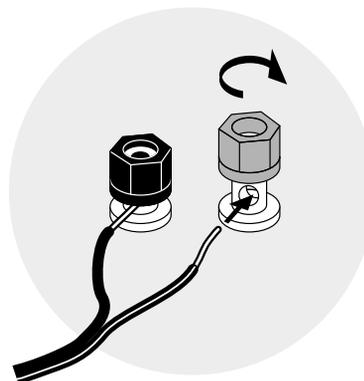
**Using the five-way binding posts:** The binding posts permit easy connection to banana plugs, spade lugs, and bare wire.
