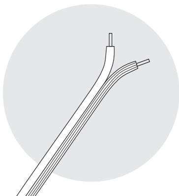
**IMPORTANT:** Typically, one side of the wire is smooth. Connect this side to the - (black) connection. The other side has a rib or stripe. Connect this to the + (red) connection.
