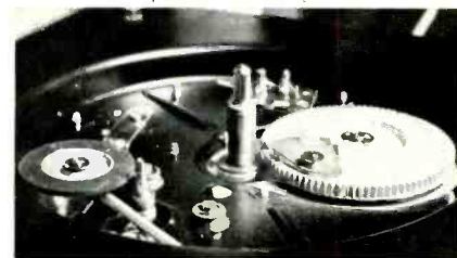
Fig. 2—View of the BSR 600 with turntable platter removed.
