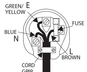
If a 13 amp (BS 1363) plug is used, a 3 amp fuse must be fitted, or if any other type of plug is used a 3 amp or 5 amp fuse must be fitted, either in the plug or adaptor, or on the distribution board.
