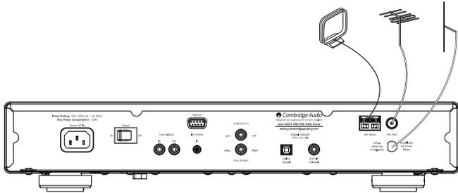
**Note:** The 651T is supplied with temporary FM or DAB aerials for initial use only. For permanent use, outdoor aerials are highly recommended.
