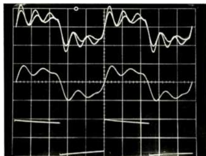
Fig. 4—Square-wave response of CAD-50SL in pentode mode at 10 kHz into 4-ohm and 8-ohm loads (overlaid traces, top), 10 kHz into 8 ohms paralleled by 2 \mu F (middle), and 40 Hz into 8 ohms (bottom). Scales: Vertical, 5 V/div.; horizontal, 20 \mu S/div. for 20-kHz traces, 5 mS/div. for 40-Hz trace.
