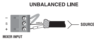
Figure 2.4 Unbalanced Input Connector Wiring
