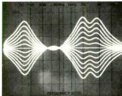
**Fig. 2—Swept-frequency responses with 63-Hz, 2-kHz, and 4-kHz filters set successively for 2-dB steps from -12 to +12 dB. Small overshoot around 300 to 600 Hz (see text) has no significant audible effect.**
