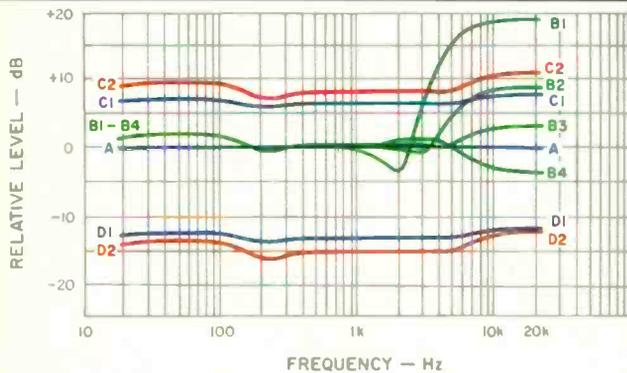
**Fig. 1—Swept-frequency response for various control settings: "Bypass" position (curve A), and with 1.5:1 expansion switched in, at four settings of the rear-panel "HF/Transition Level" pot (curves B1 through B4). With input level raised 5 dB, mid-frequency level rises 6.5 dB with 1.3:1**
