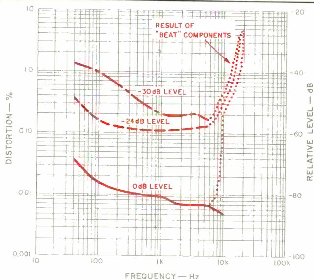
**Fig. 3—THD vs. frequency at three signal levels.**
