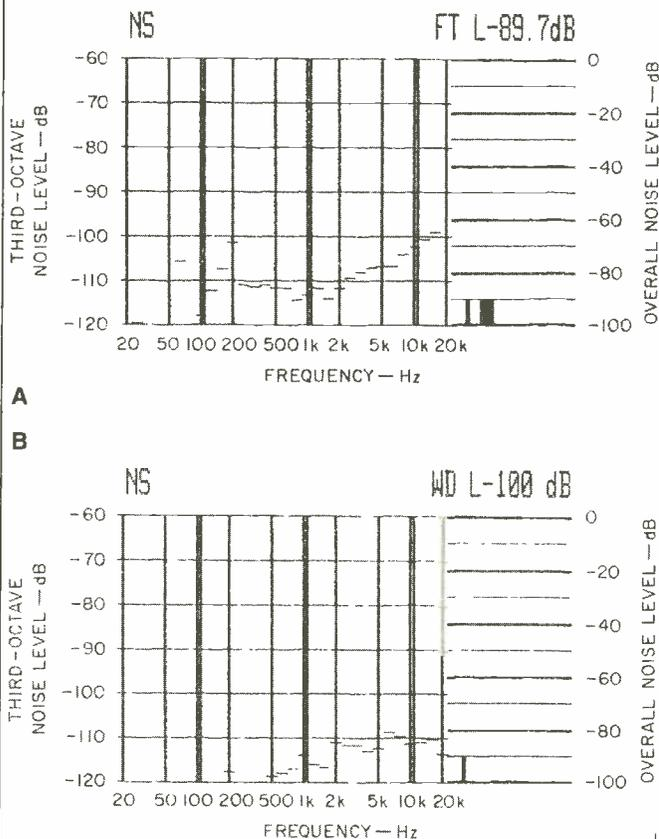
**Fig. 2—Signal-to-noise analysis, unweighted (A) and A-weighted (B).**
