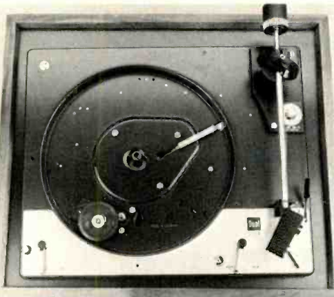
Fig. 5 —Top view of the unit with the platter removed, showing the simplicity of this side of the chassis. The idler wheel, shown at the lower left of the turntable well, retracts from the stepped and tapered motor shaft when the STOP position.
