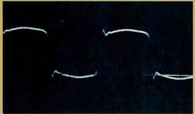
Fig. 2 — Square wave response, Ortofon ULM 60E cartridge.
