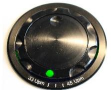
As soon as the desired speed is reached the LED glows white permanently.
