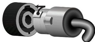
To connect the Jazzmaster™ Ultralight speaker to an Ultralight amplifier, use the Speakon® cable included with the amplifier. Rotate the Speakon® connector to align it with the input slots, then fully insert the connector.
