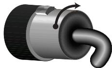
Rotate the connector clockwise until it locks into place.
