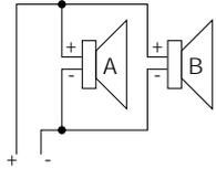
\*Example- Cabinet A is 8 ohms. Cabinet B is 16 ohms. The total impedance when connected in parallel is:
