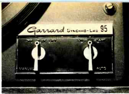
Fig. 5—Combined manual-cueing-pause control is shown at left; automatic control lever at right.
