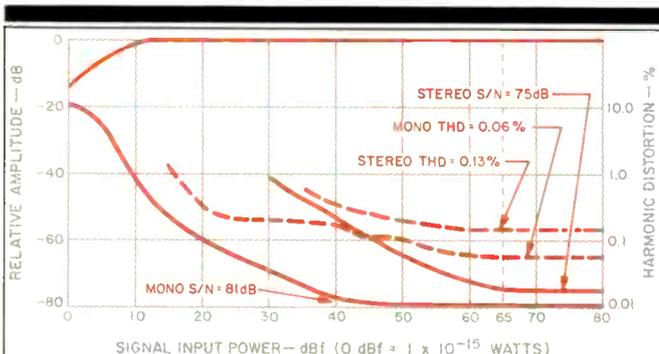
Fig. 1—Mono and stereo quieting and distortion characteristics.
