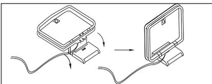
6. Connect the supplied FM antenna to the **FM (75-ohm) Connection 41**. The FM antenna may be an external roof antenna, an inside powered or wire-lead antenna or a connection from a cable TV system. If the antenna or connection uses 300-ohm twin-lead cable, you must use the 300-ohm-to-75-ohm adapter supplied with the unit to make the connection.
