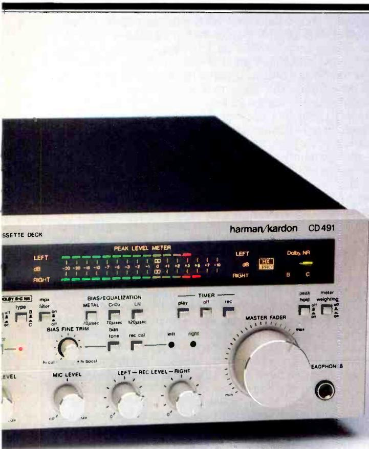
switch is pushed in, the reverse of what I had expected. Just below the NR pushbuttons is the tape monitor switch, which latches in for tape playback, turning on a red LED at the same time.
