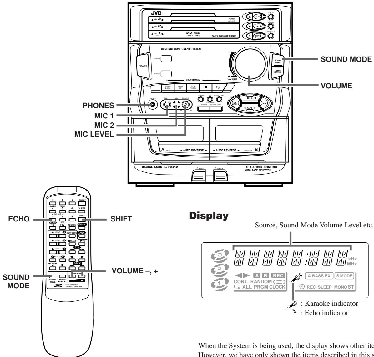
When the System is being used, the display shows other items as well. However, we have only shown the items described in this section.
