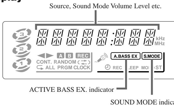
When the System is being used, the display shows other items as well. However, we have only shown the items described in this section.
