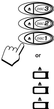
**1. Press the  $\blacktriangle$  button on the left of the Disc button you want to insert the disc into.**
