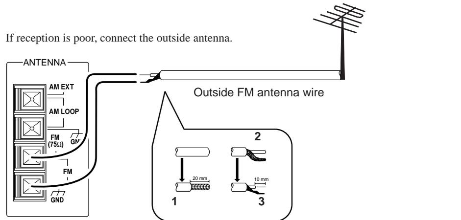
Before attaching a 75 ohm coaxial lead (the kind with a round wire going to an outside antenna), disconnect the supplied FM Wire Antenna.
