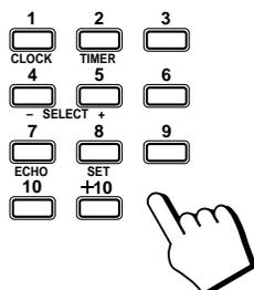
The preset number appears in the display after you have pressed the number keys. If the key is pressed continuously, the preset number display blinks. Release the button after the number starts to blink. This completes the preset setting.
