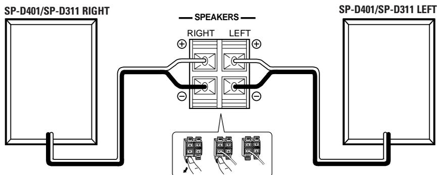
**IMPORTANT: Use speakers with the correct impedance only. The correct impedance is indicated on the back panel.**
