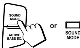
**To get an effect,** press the SOUND MODE button repeatedly until the Sound Mode you want appears in the display. The frame around the “S.MODE” indicator lights up.
