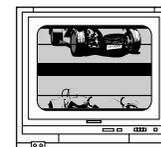
Picture turbulence due to sync unmatching.
