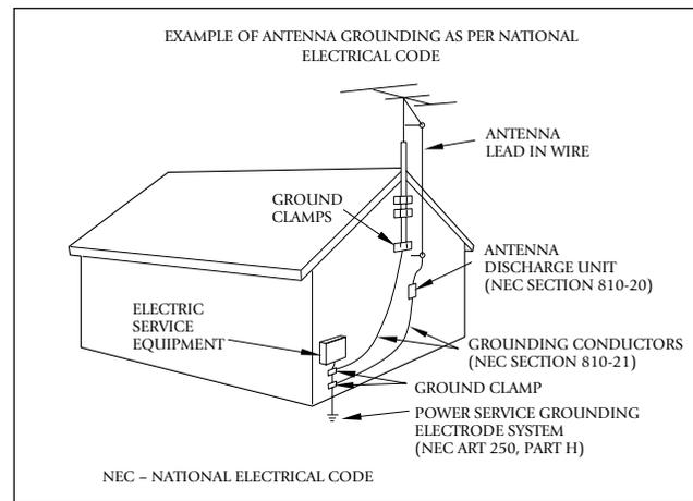
**18. Power lines** – An outside antenna system should not be located in the vicinity of overhead power lines or other electric light or power circuits, or where it can fall into such power lines or circuits. When installing an outside antenna system, extreme care should be taken to keep from touching such power lines or circuits as contact with them might be fatal.
