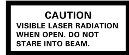
Inside this laser product, a laser diode classified as Class 2 laser radiation is contained as alerted by the internal caution label shown above. Do not stare into beam.
