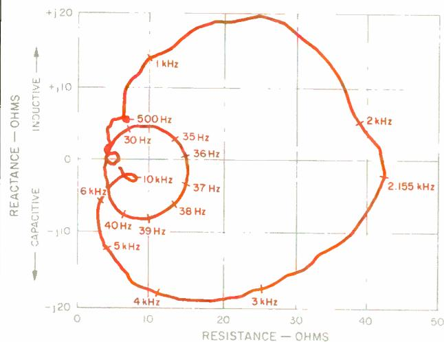
**Fig. 3—Complex impedance. Note the rescaling from Fig. 2.**
