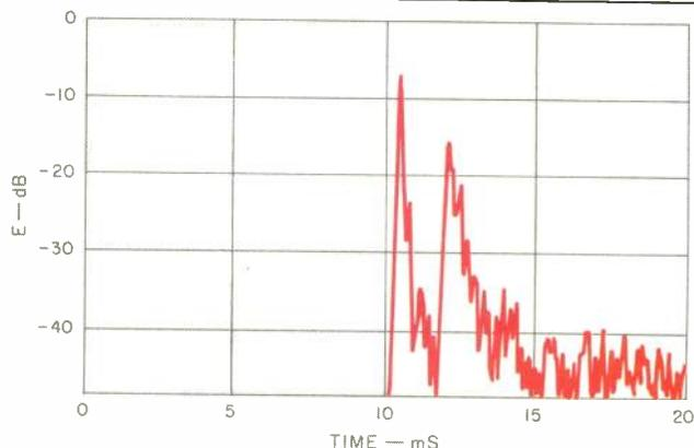
**Fig. 7—ETC of Fig. 6 minus the room reflections.**
