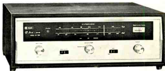
Fig. 1. The Knight-Kit KG 790 tuner shown in its optional walnut enclosure.
