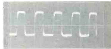
Fig. 9—Square-wave response at 100 Hz (A) and 10,000 Hz (B).
