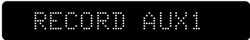
If you want to record a different source than the one currently selected, press the corresponding source selection button; the Display will then show the input number of that source (for example, **RECORD DBS2**).
