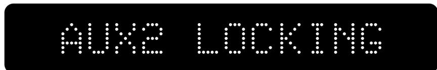
If no digital signal is present (if the source is turned off, is improperly connected, or is disconnected), this part of the Display will show:
