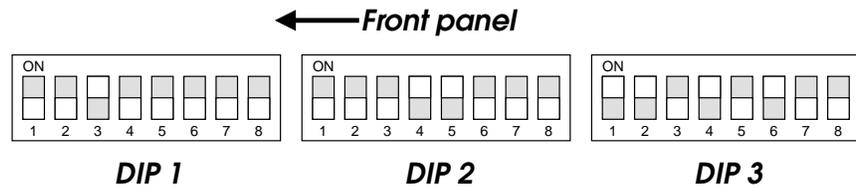
Each of these DIP switches' eight miniature switches corresponds to digital inputs 1 through 8. To assign an alias to an input, you must set the corresponding miniature switch to the proper position on each of the three DIP switches.
