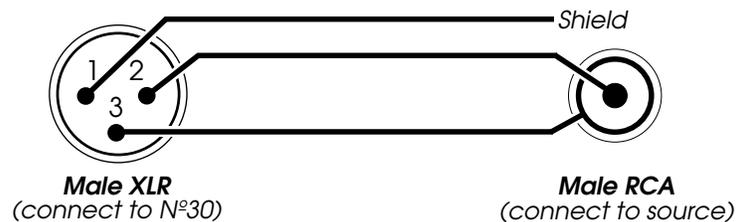
If using a two-conductor 75Ω cable, including a 237Ω resistor as close as possible to the XLR termination may, in some cases, improve sonic performance; follow the diagram below.
