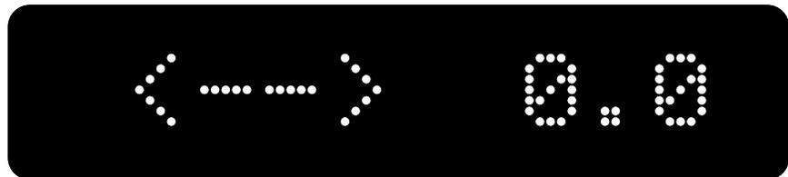
Turning the Output Level control in either direction will change the balance in that direction. The display will reflect this by changing to the appropriate single-headed arrow to indicate the direction of change and by showing the number of decibels by which that channel has been increased (in tenths of a decibel), as below:
