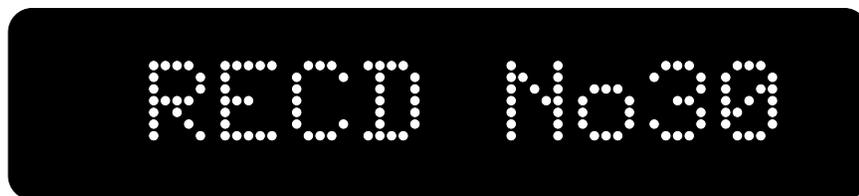
To select a different input for recording, simply press the appropriate Input Selection button while in this mode. Note that the N°38 will not allow a recording device to serve as its own source while monitoring itself, as this would allow potentially dangerous feedback to be reproduced by the loudspeakers. (See "Programming Input Aliases" for more details.)
