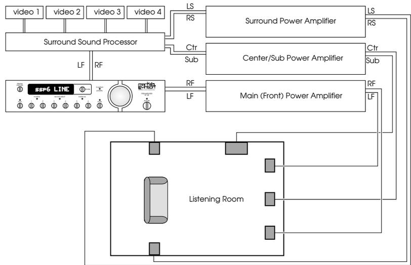
**Note:** the N°38 will not allow an input with an "ssp" alias to be selected during initialization, since allowing a line level signal to pass through unattenuated at start-up presents a potential hazard to your loudspeakers.
