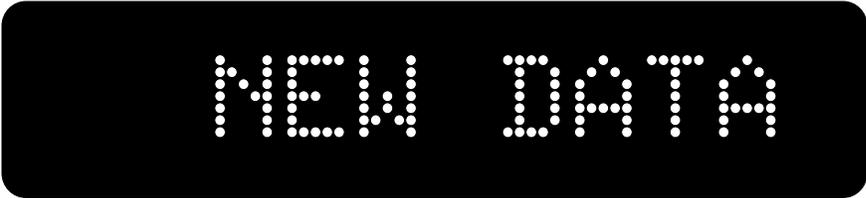
This indicates that your new **Automatic Output Level** has been stored in non-volatile memory. Your N°38 will now automatically return to this volume setting whenever this input is selected. To reverse this situation, simply re-adjust the **Input Offset** as described above (in "Programming Input Offsets").
