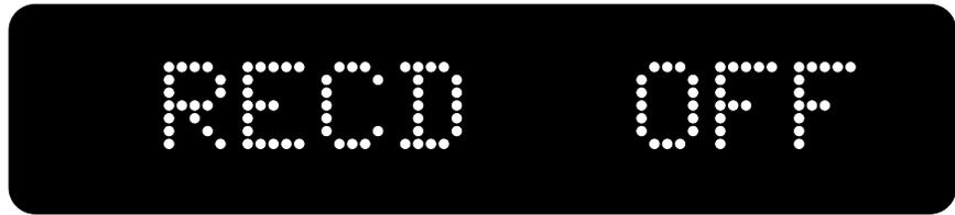
Defeating the Record Outputs eliminates even the possibility that the input impedance of a recording device could have an effect on the sound quality of the preamplifier. We recommend that Record Outputs be turned OFF when not in use.
