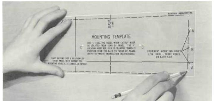
If the cutout is to be located from the front of the panel, begin at step 2. If the cutout is to be located from the rear of the panel, begin here.
