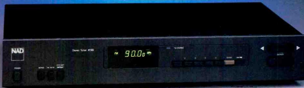
The name Larry Schotz has been associated with FM tuner products produced and sold by NAD ever since that company delivered its outstanding 4150 tuner some two years ago. The new NAD 4155 incorporates a new concept developed by Mr. Schotz, which NAD calls Dynamic Separation. Basically, this circuit reduces noise normally heard during weak-signal stereo FM reception by blending the highs during quiet moments or pauses in the music (when background noise would be most obvious and obtrusive)
