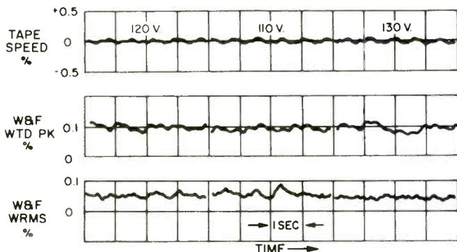
Fig. 6 — Wow and flutter (three trials) and tape play speed vs. time and line voltage.
