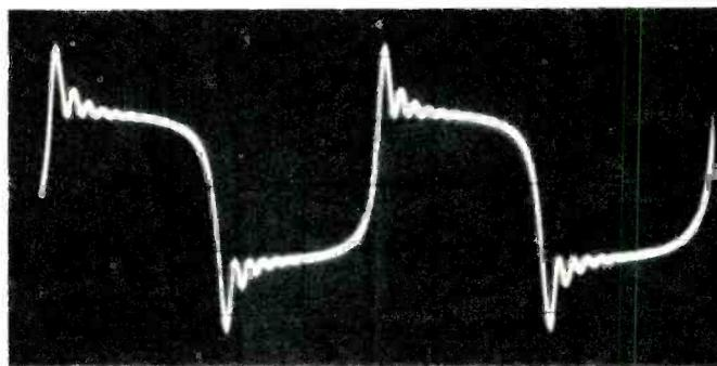
Fig. 7 — Record/playback of a 1-kHz square wave.
