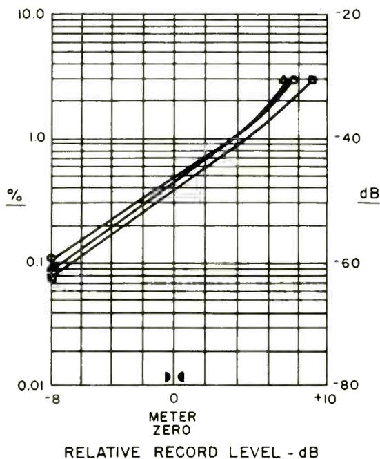
Fig. 5 — Third harmonic distortion vs. level in Dolby mode at 1 kHz with Nakamichi EX-II, SX, and ZX tapes.
