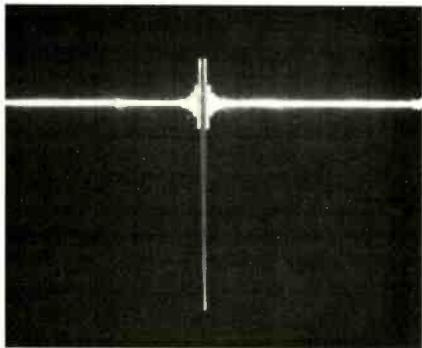
Fig. 8—Single-pulse test.
