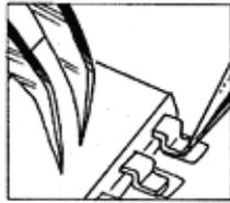
*Secure the IC and solder.*
