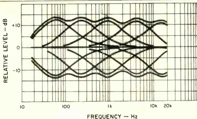
**Fig. 1** — Swept-frequency responses with and without EQ; controls flat, each at maximum boost and also cut individually; all controls at maximum boost and at maximum cut. (Bandwidths set at maximum, 1.6 octaves.)
