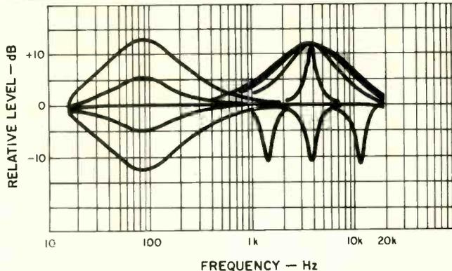
**Fig. 2** — Response with lowest filter set to maximum bandwidth and 90 Hz, and gain control set to -12, -6, 0, +6, and +12, successively. Responses with 4-kHz filter at maximum boost with four bandwidth settings, and at maximum cut and minimum, center, and maximum frequency.
