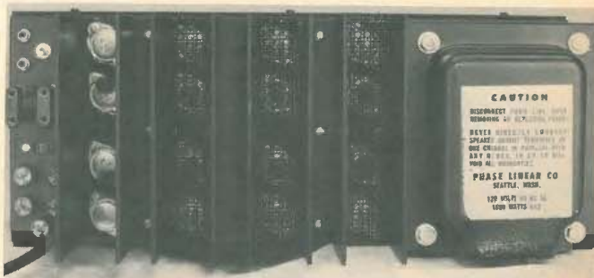
Fig. 1—Rear view of the amplifier with one protective perforated metal shield removed from one group of transistors. All input and output connections are made at the left end of the unit.
