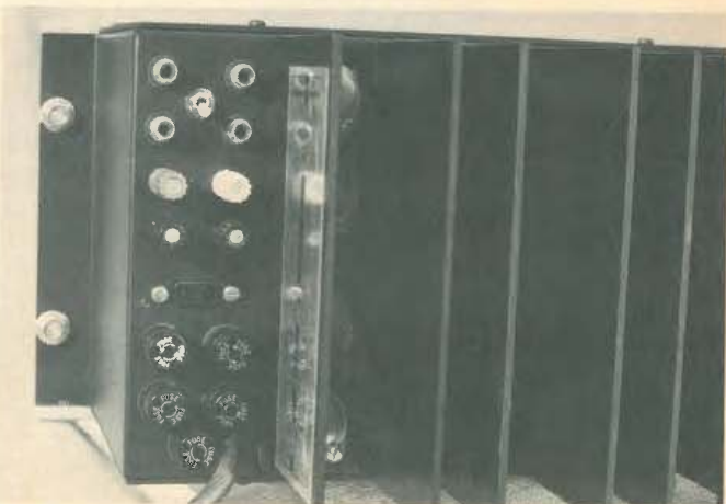
Fig. 2—The terminal panel with normal inputs at top, direct inputs immediately below, together with selector switch. Then come the four heavy-duty binding posts, an a.c. receptacle, four d.c. supply fuses, and the a.c. line fuse and line cord.
