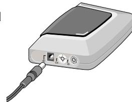
*Note* To avoid interference, the adapter cable should be kept away from the RF Extender as far as possible.
