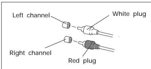
Connect the TAPE jacks of your amplifier to the LINE jacks of the cassette deck. Be sure to connect the REC (INPUT) jacks of the deck to the recording (output) jacks of the amplifier, and the PLAY (OUTPUT) jacks of the deck to the play (input) jacks of the amplifier.
