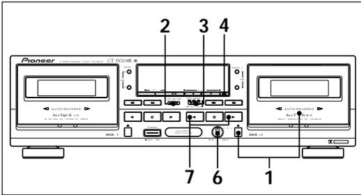
1. Load a tape for recording in Deck II.
