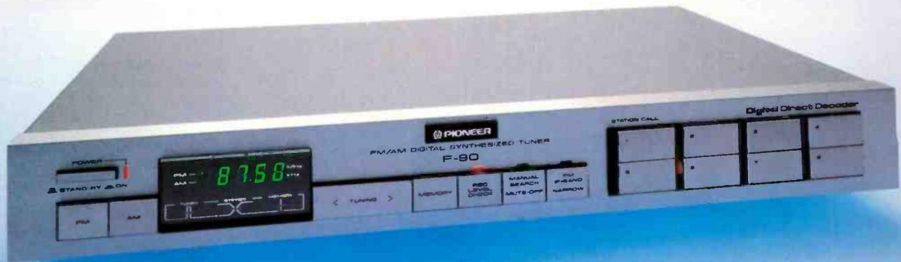
The most outstanding feature of this new AM/FM tuner from Pioneer is its Digital Direct Decoder, a unique system which decodes stereo directly from FM i.f. signals instead of having to decode the composite signal appearing at the output of the FM ratio detector or discriminator. The new circuit is said to improve overall sound quality of FM reception, particularly in the areas of stereo separation, distortion and signal-to-noise ratio.
