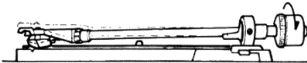
Headshell end is too heavy – Turn the counterweight in the direction of the arrow.
